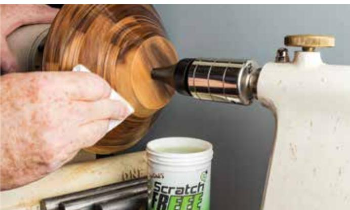
A wax with fine abrasive compound mix being used to refine a finished surface
