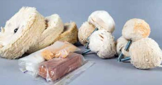
There are many sizes, shapes and grades of buffing wheel available alongside myriad forms of abrasive and finishing compounds to apply to the wheels. For manipulating or applying finishes, loose-fold wheels are most commonly used
