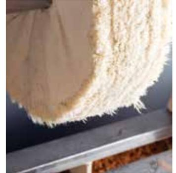
It is best to dress, also known as conditioning, the wheels with a wire brush or special toothed comb prior to loading or charging the wheel with a finish or abrasive compound. Charging the wheel is best done lightly and as needed. Always err on applying too little rather than too much abrasive or finishing compound on a wheel
