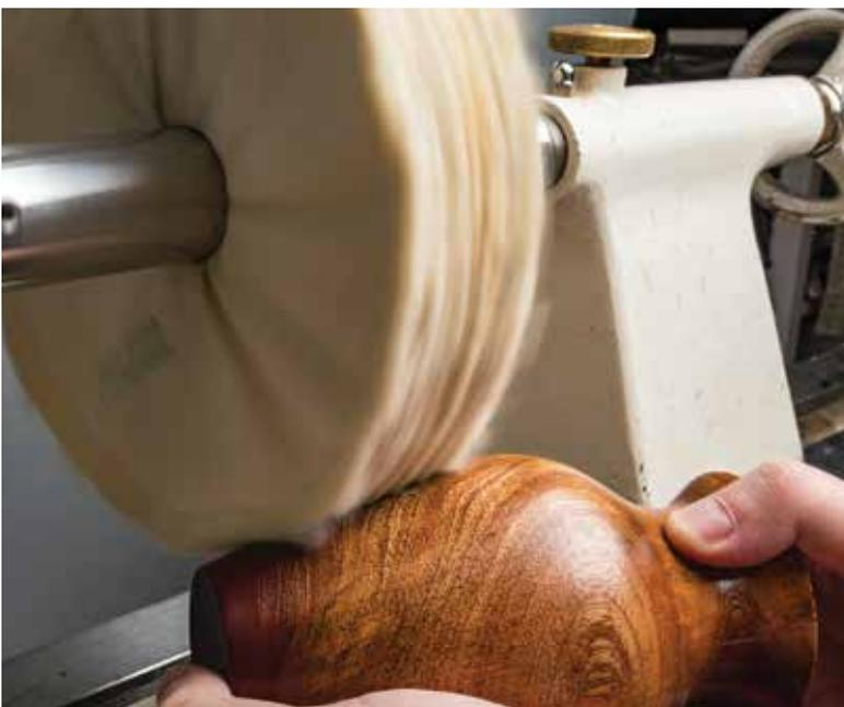
If you want, manipulate an applied finish on the work with a fine abrasive compound and, if desired, follow this by using a wheel or buffing pad loaded with a wax compound or finish to achieve a glossy effect
