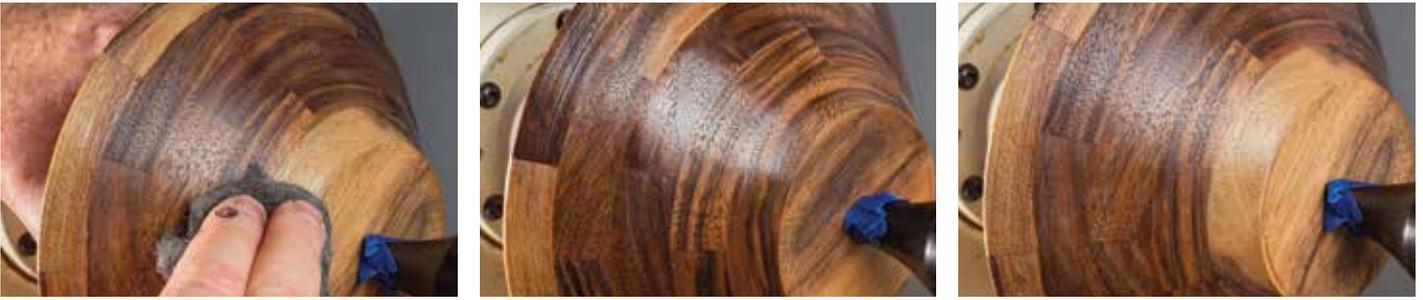
Using 0000 steel wool dry with soft circular motions takes little effort take any high gloss back as desired to any desired level down to matt
