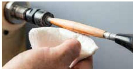
With the lathe off, wipe on your thin CA application axially then rotate by hand to cover entirely
