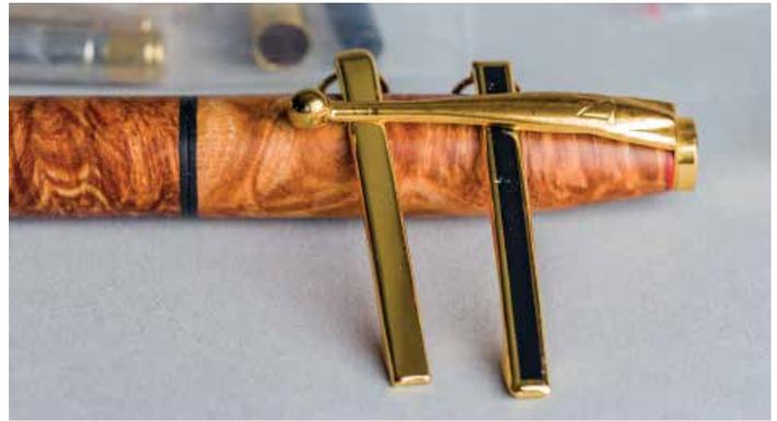
The most noticed difference in the quality of the kits is the construction of the clip. Durability also varies
