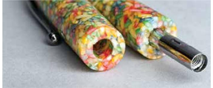
You can also make up the lost length and more if desired by leaving part of the interface ends partially unsupported by brass tube
