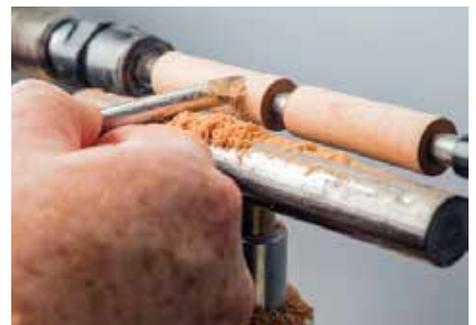
A ground discount store screwdriver illustrates that a properly sharpened and presented tool will cut wood very nicely. This is done just to prove a point – don't do this at home, buy correctly made blades
