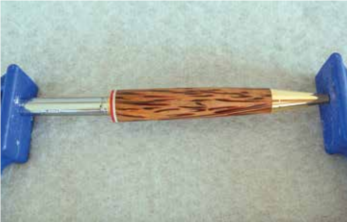
A bench clamp can be used for assembly. Take the rubber cushions off
