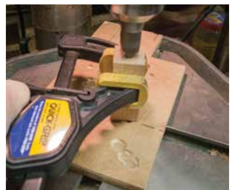
Using a slow speed and piloting on the tube I.D., the pen mill will create a perpendicular face
