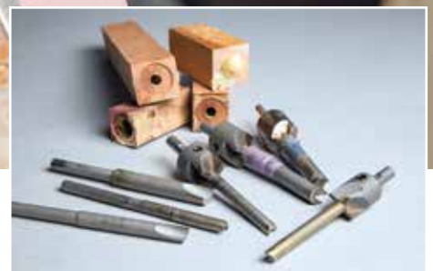
Pen mills are available with different pilot sizes. I often use tape in a pinch
