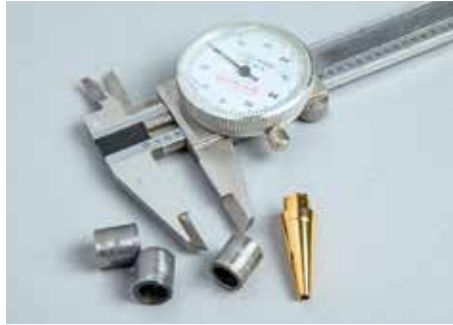
Parts and bushings vary in size. Bushings will continue to get smaller with sanding
