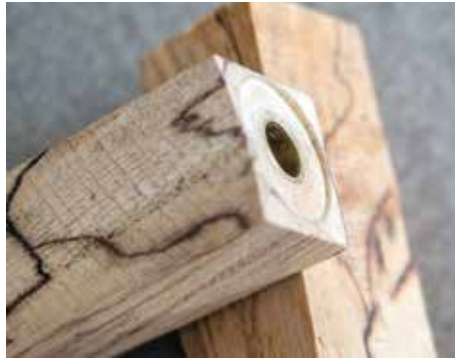
The facing should only be deep enough to expose the end of the brass tube
