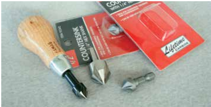
Chamfer tools are available from machine tool grade to bargain basement. They all work fine
