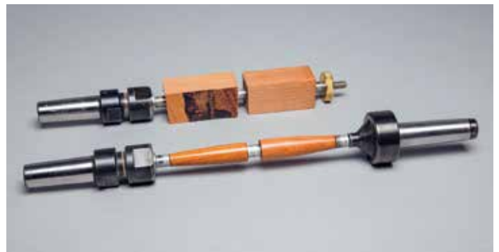
A mandrel saver swallows the shaft putting all of the force on the bushings and brass tubes
