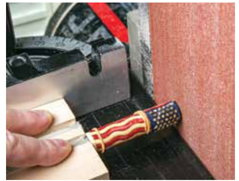
Alternatively, piloting on the I.D. of the tube and sanding will face the blank
