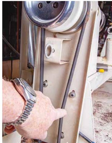
**Whether regular V or poly V belt, there needs to be a bit of flex. Finger pressure mid-belt should deflect it slightly when tensioned properly**
