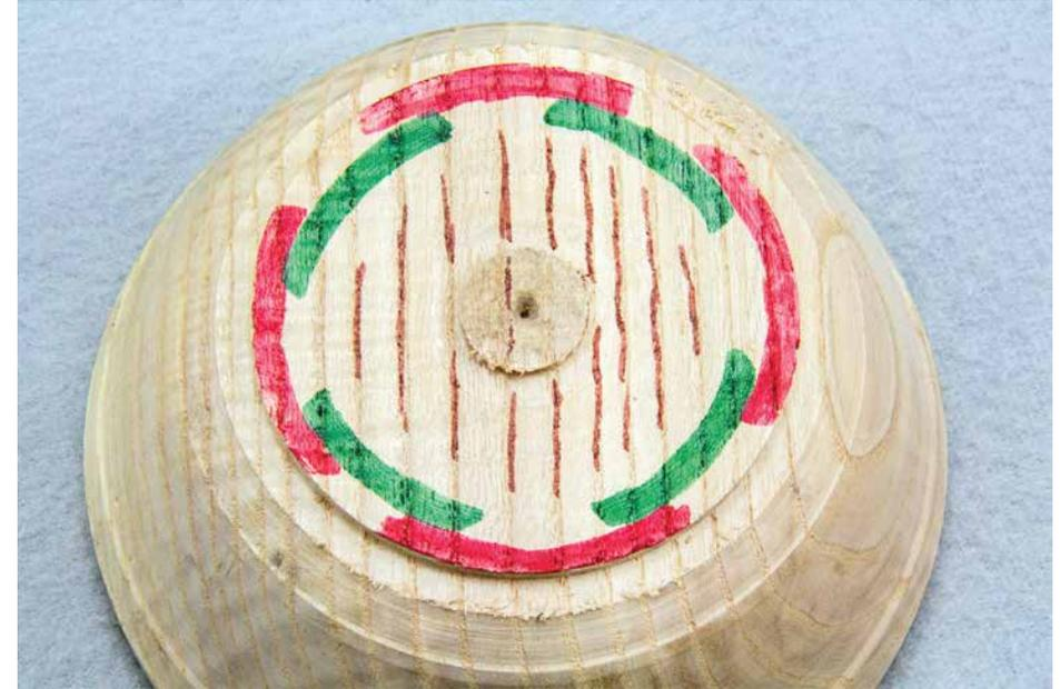
**The best strength and durability for clamping on a tenon is with the chuck jaws angled to the grain (green) as opposed to on axis and across the grain (red)**
