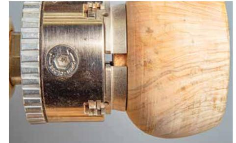
**Good practice for chuck mounting is to mount flush on the tenon shoulder with a good tenon depth, without touching the bottom of the chuck**
