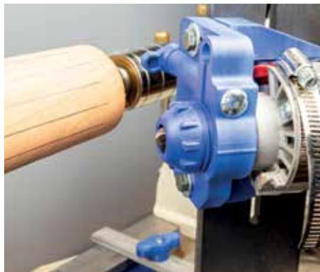
The mini router tool holder works superbly with my Bosch Colt router. Plenty of available cutters and curve tracking nose with superb depth control
