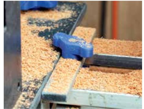
Longitudinal travel limits for fluting are easily set with the provided stop clamps on the lathe bed
