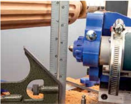
The Flutemaster centerline cutter height can be adjusted from under 4in to over 12½in covering every lathe you'll likely use
