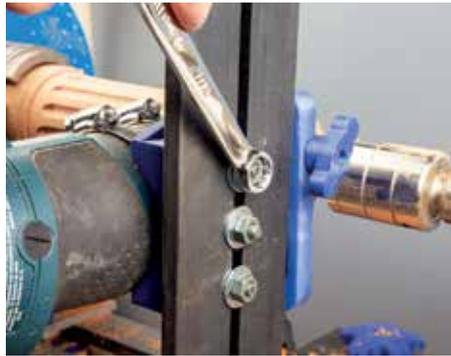
The only tool required for changeover to another sized lathe is a single wrench. Only requires attention to set the cutter on the centerline axis
