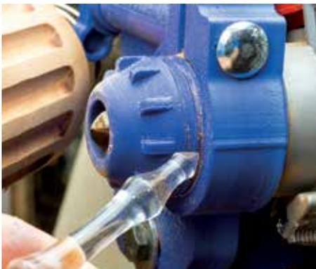
The depth control resolution is marked off in .002in per tick mark. Easily set and locked in place for precise control and repeatability
