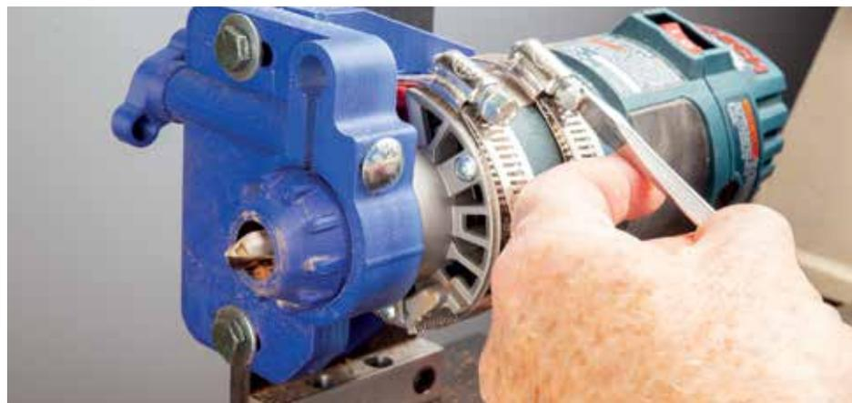
The available tool holders are 3D printed parts. Fully functional yet less expensive than metal fabrications help moderate selling price
