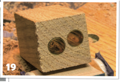
18 I'm a huge fan of a compliant adhesive such as polyurethane to fasten the brass tubes into my pen blanks. Planning helps with cure time 19 Don't be afraid to give some thought to how much clearance you would like for adhesive between the tube and the blank
