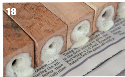
18 I'm a huge fan of a compliant adhesive such as polyurethane to fasten the brass tubes into my pen blanks. Planning helps with cure time 19 Don't be afraid to give some thought to how much clearance you would like for adhesive between the tube and the blank
