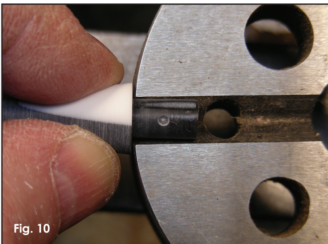
A removable nib benefits from a shallow dimple for gluing.
