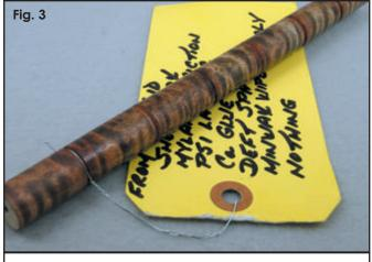
A test piece to compare various finishes tried over an experiment in dyeing wood.
