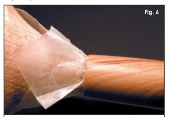
Waxing bushings isn't my way, so I use waxed paper on my own tapered mounts, which I use for turning as well.
