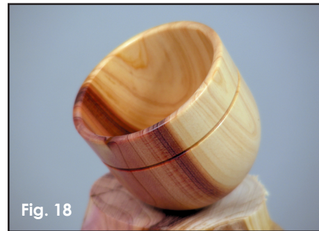
Fig. 18 The scoop body completed with the mounting wire groove cut.
