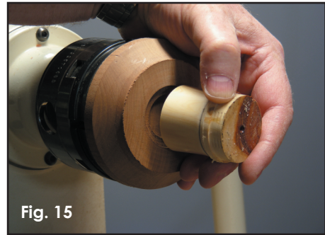
Fig. 15 A scrap mounted in the chuck; a jam chuck is created to hold the scoop blank.
