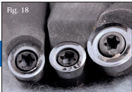
The #1 Osprey (left) and the #1 Mini Hercules (center) share the same carbide cutter design bedded at different angles; the #2 Osprey (right) cutter is much larger in size. The Ospreys have round tool shafts, while the Mini Hercules has a square tool shaft.
