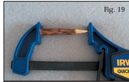
Though a drilling vise or a pen press can be used to assemble a pen, so can a quick clamp, if the rubber bumpers are removed to allow the plastic faces to contact the pen parts.
