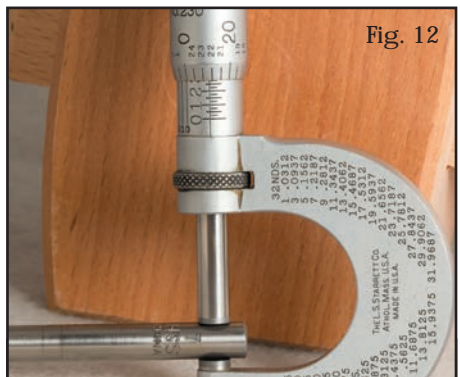
Fig. 12 Whether high priced or economy priced, the indicated size on the drill is rarely the actual size. All have a manufacturing tolerance, with some more than others. Here a 7mm drill actually measures 0.272".
