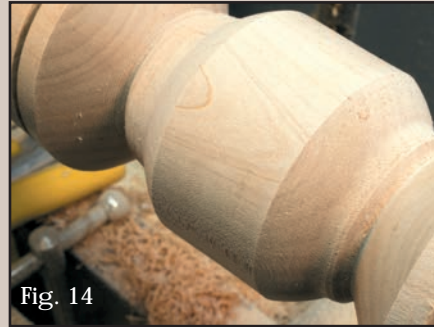
Fig. 14 The diameter that is in the center where the shear scraping took place exhibits excellent surface finish. Though sanding could improve it, there is no evidence of any tearout to deal with.
