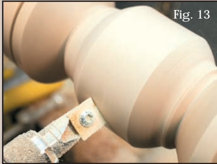
Fig. 13 Rotating the cutter 45° and performing a shear scraping produces far better results. The very fine curls are indicating that the surface will be in excellent shape.
