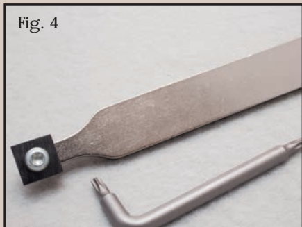
There is a cutter holder allowing for sharpening of the cutters on a grinder. The life of the replaceable cutter can be extended for additional economy.
