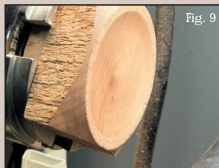
As expected, the end-grain scraping with the cutter in the flat position leaves a certain amount of torn-out grain. This is not unlike any other scraper used in this manner.
