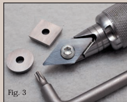
Fig. 3 All the cutter tools that are available fit into the head and are fastened with a Torx head screw. The position of the various cutters allows for them to be used with support underneath the majority of the cutter.
