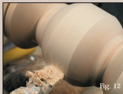
Whether creating a tenon for a chuck mounting or scraping the outer diameter, the flat scraper really doesn't work well with the grain in this piece.
