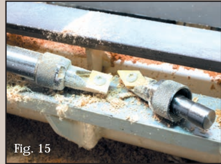
Fig. 15 The rotation of the heads is quick and easy. The changing of the cutters is not as quick. You might want to consider buying additional heads to keep different cutters in for speed of change.
