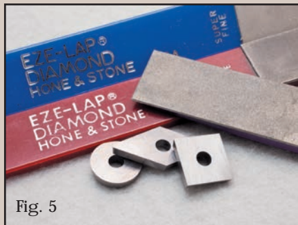
The carbide cutters can have their life extended for a period of time by touching up with a diamond hone. They have a finite life, but it can be extended with continued care.
