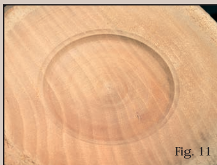
The inner ring where the shear scraping took place gets the torn-out grain cleaned up in contrast to the outer diameter that was flat scraped only.
