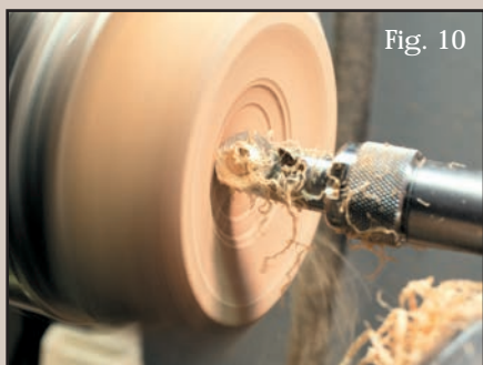
The cutter is rotated 45° left and then the tool is used as a shear scraper. It creates much finer shavings and cleans up the torn-grain area.
