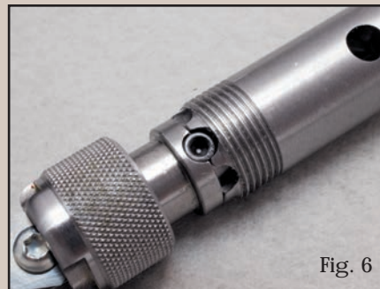
Shown with the lock ring unfastened, the three different positions available to the user are flat, 45° left, and 45° right. Once positioned, the lock ring secures the head.
